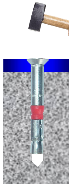
Insert assembled anchor through fixture into concrete
